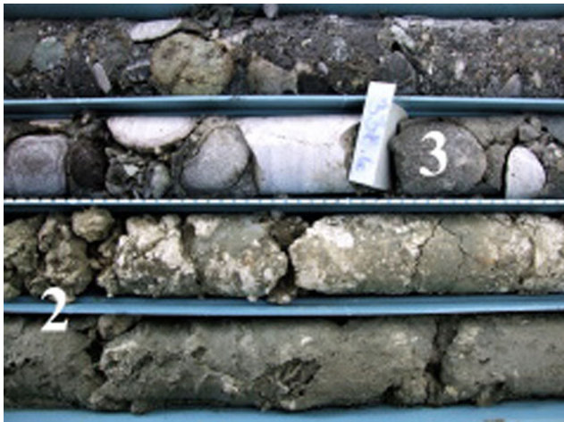
Fig. 6. Two sequences (2 and 3) from the alluvial-lacustrine facies (RTK-1502A); 2, The top of this sequence is represented by fine-grained clastites with concretions of carbonates (white-bead bark of decomposition); 3, Polymict gravel in the base of sequence.
