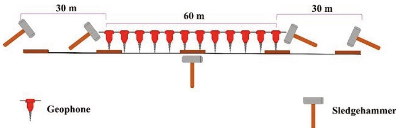
Fig. 4. Acquisition of refraction seismic.
