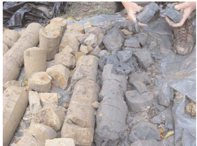
Fig. 7. A view on the archaeological layers (left) and the new the Plio-Pleistocene unit (right) in the borehole V-2 (courtyard of the archaeological site).
