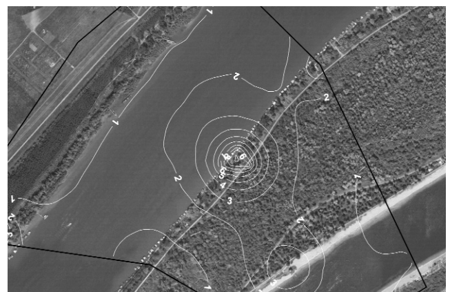
Fig. 4. Piezometric head difference between lower and upper layers (floor, roof, and interlayer).
