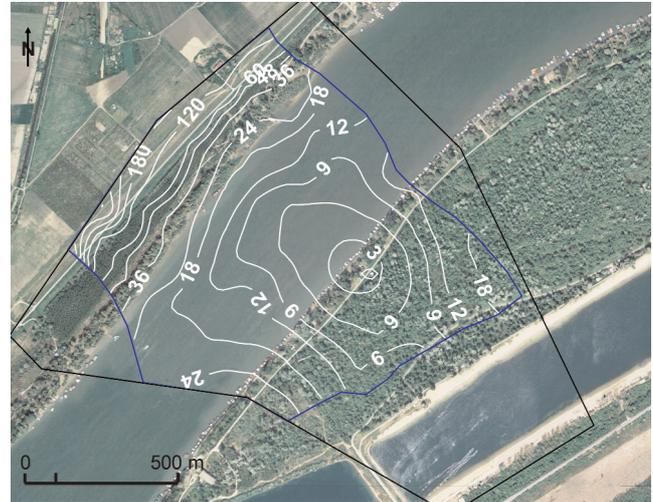
Fig. 8. Time zones of groundwater travel through the semi-permeable interbed (in months).
