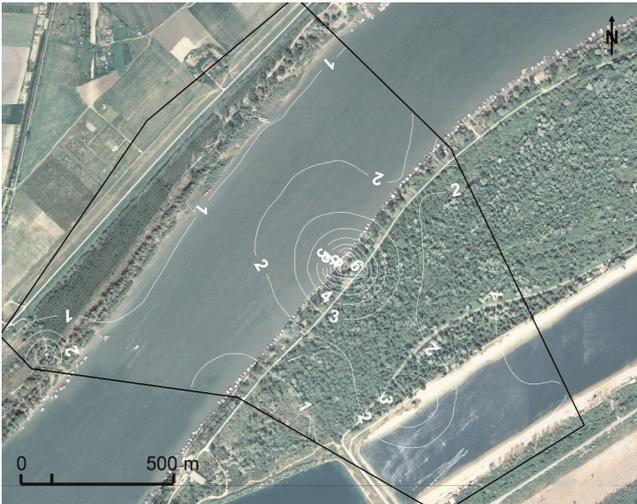
Fig. 6. Piezometric head difference between the lower and upper layers (interbed floor and roof).
