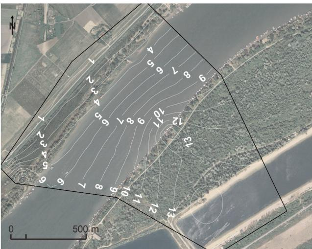
Fig. 11. Piezometric head difference between the lower and upper layers (interbed floor and roof), at reduced interbed conductivity ( $K_{vert} = 1 \times 10^{-9}$  m/s).
